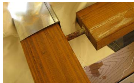
Slip the center pole pins through the pre-drilled holes in the ridge pole. (See Step 5.)
