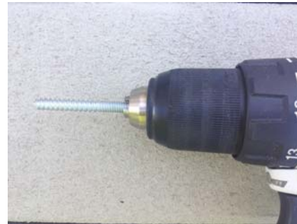
Hanger bolt with nylon wing nut. Place the hanger bolt directly into the drill chuck. (Step 9.)
